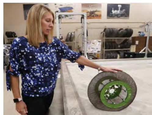
Heather Oravec rolls a nickel titanium Shape Memory alloy tire on a simulated extraterrestrial surface in a lab at NASA Glenn Research Center in Cleveland. Photo: Mike Cardew/Beacon Journal/Ohio.com
